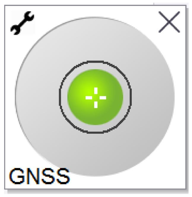
The circle on the **eBubble** vial represents the configured tilt tolerance. **Tilt tolerance** is defined as the distance on the ground **(tilt distance)** that the tilt represents given the antenna height:
