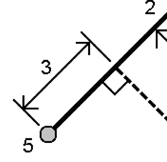
The distance along the line (3) and the perpendicular distance (4) to the line is calculated. The distance along the line is from the point specified (5).
