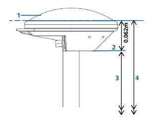
**NOTE** – If this antenna is mounted on a tripod, measure the height from the ground mark to the top of the notch protruding from the side of the antenna.
