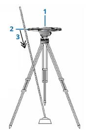
**NOTE** – Measure the height to three different underside notches around the perimeter of the groundplane. Then record the average as the uncorrected antenna height.
