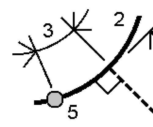
The distance along the arc (3) and the perpendicular distance (4) to the arc is calculated. The distance along the arc is from the point specified (5).
