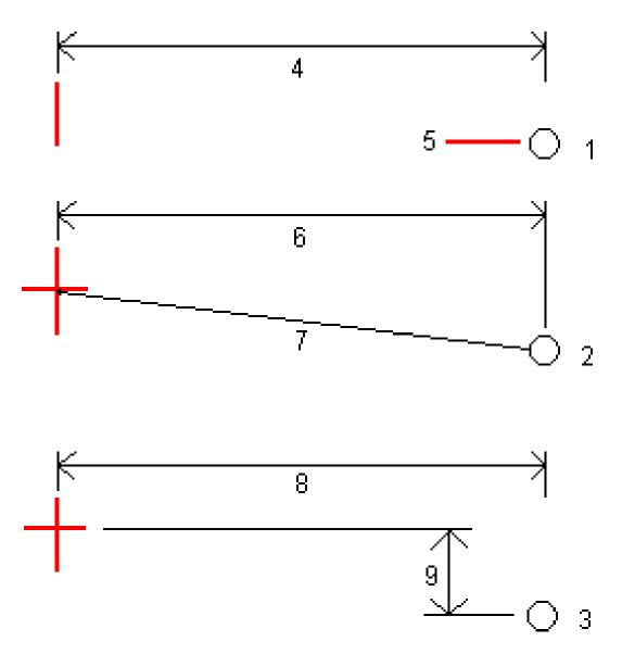
**1** – **Offset and elevation**. Enter an offset **(4)** from the polyline, and the elevation **(5)** of the hinge position.
