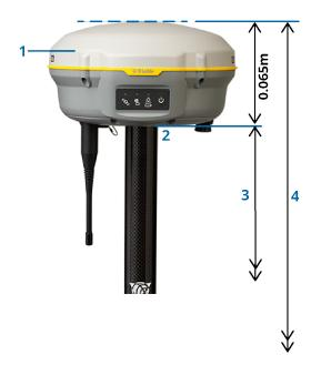
**NOTE** – If this receiver is mounted on a tripod, measure the height from the ground mark to the center of the yellow bumper between the gray base and the white top of the antenna, and select **Center of bumper** in the **Measured to** field. Note this is a slope measurement.
