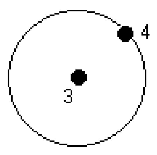
Measure a single point (1) at the center of the circle where that point uses the Start circle (center) control code and the line feature code, followed by a radius value (2). For example, <Start circle (center)> <Line feature> 8.
