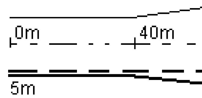
If you select an offset/string that has an offset value of 5 m, the offset value updates to follow the solid line for subsequent stations. In this example, the offset changes from 5 m to 8 m between stations 40 m and 100 m and then is maintained at 8 m for subsequent stations.
