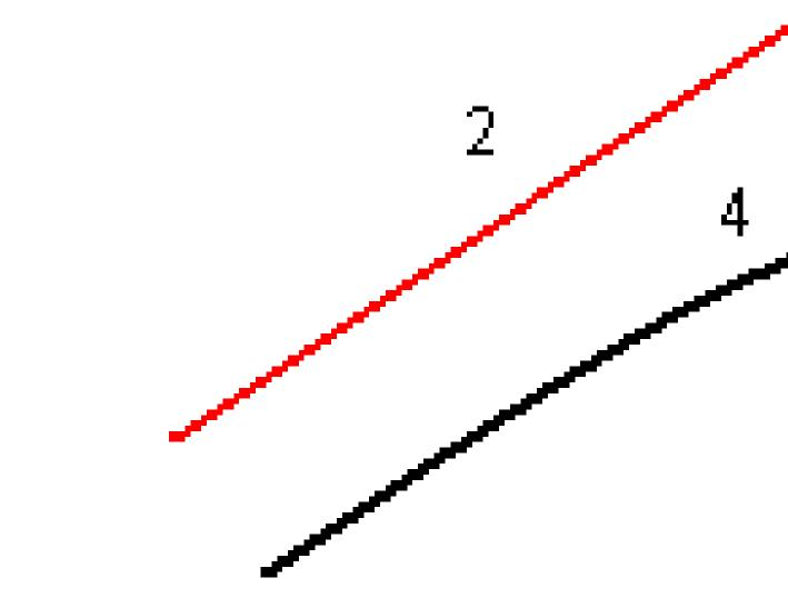
When staking stations on a string, you can define a horizontal offset by the distance from the selected position to the alignment. To do this:
