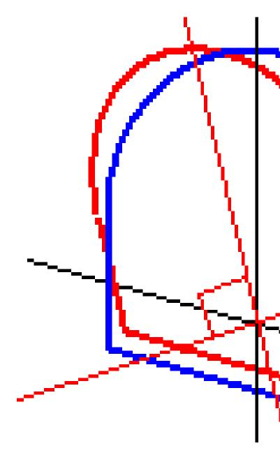
The station and offset display of points relative to a tunnel using **Point manager** or **Review job** are only calculated vertical to the alignment. If the templates were applied perpendicular in Tunnel positioning then the station and offsets will be different.
