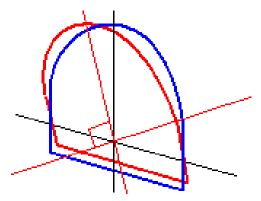
The station and offset display of points relative to a tunnel using **Point manager** or **Review job** are only calculated vertical to the alignment. If the templates were applied perpendicular in Tunnel positioning then the station and offsets will be different.
