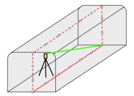
Previously the software staked out the centerline only along the mine roof.
