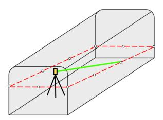
Previously the software staked out the gradeline along a single mine wall only.
