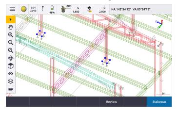
Objects in IFC files can be displayed as solid objects with 100% opacity; you can reduce the opacity or display as a wireframe. To make the object more transparent, or to view the model as a wireframe rather than a solid object, tap and select **Settings** and then modify the options in the **IFC** group box.
