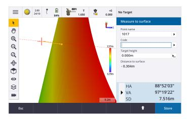
During measurement, the closest position on the surface is highlighted in the map and a line is drawn from the measured position to the position on the surface. The **Distance to surface** value and the coordinates of the closest point on the surface are stored with the measured point and can be viewed in Review job and Point manager.
