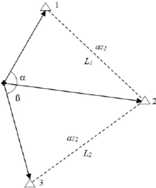
with: 3 observed control points 1, 2 and 3 (coordinate values  $X_1, Y_1, X_2, Y_2, X_3, Y_3$ )
