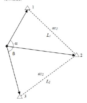
with: 3 observed control points 1, 2 and 3 (coordinate values  $X_1$ ,  $Y_1$ ,  $X_2$ ,  $Y_2$ ,  $X_3$ ,  $Y_3$ )
