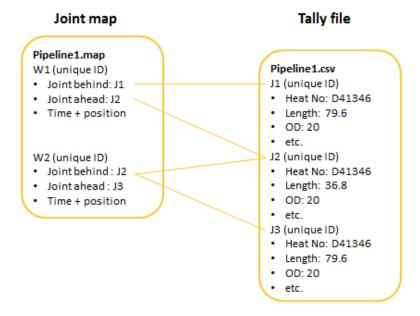
In this example, the weld W1 is linked to the joints J1 and J2. If required, the details for J1 and J2 can be updated during joint mapping and the changes are saved in the tally file.
