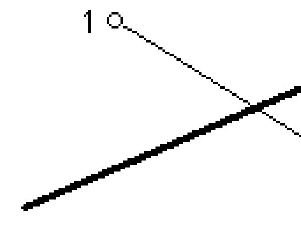
From the map, select the two points (1) and (2) that define the object that crosses the pipeline. If they are not already either side of the pipeline, these two points are projected to determine the crossing point for the object.
