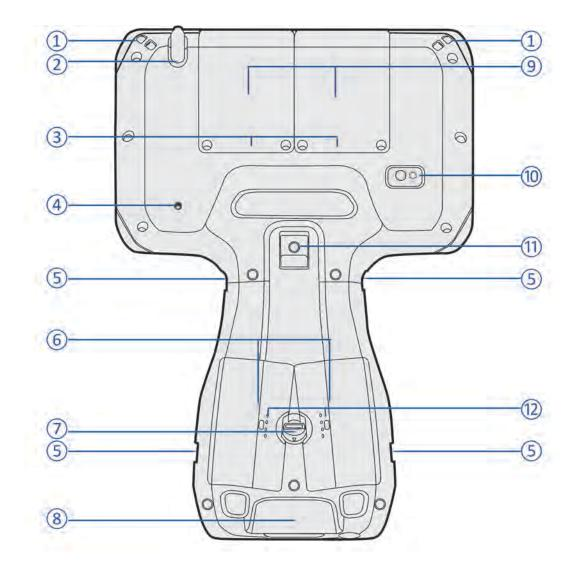
1 Stylus Tether Points 7 Battery Lock 2 Stylus bay 8 Swappable / Replaceable I/O Boot 3 SD and SIM Card Slots, behind Modules / 9 EMPOWER Module Bays (x 2) Module Bay Covers Camera - Rear, 8 MP, Auto-Focus 4 Stylus Bay Drainage Hole 10 5 Handstrap Connector Points 11 Pole Mount Latch 6 Hot-Swappable, Field-Swappable, Long Life 12 Battery LEDs Battery Pack (2 x Batteries)
